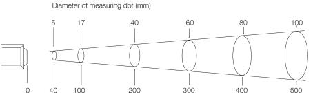
Distance between sensor and object (mm)
