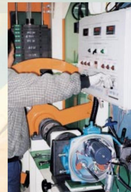
Torque Test of Actuator
