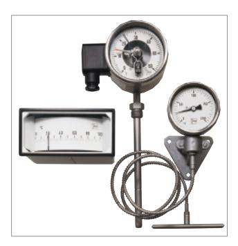
A version filled with glycerine is available as an option for service at measuring points exposed to strong vibrations. The fill dampens the measuring system when exposed to mechanical vibrations and thus enables steady indication; it also provides good lubrication for moving parts.
